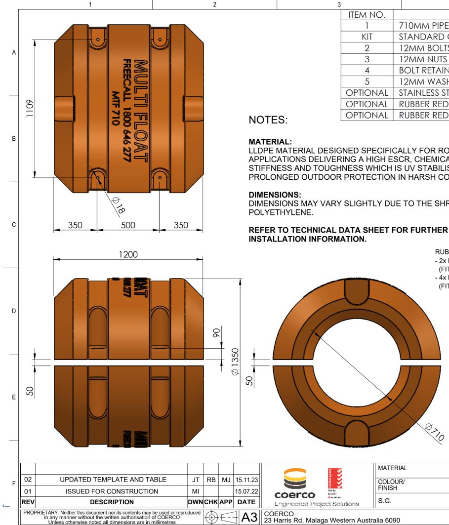
5 DESCRIPTION 710MM PIPE FLOAT SET STANDARD GALVANISED FASTENER KIT INCLUDES: 12MM BOLTS 12MM NUTS BOLT RETAINER INSERTS 12MM WASHERS STAINLESS STEEL FASTENER KIT RUBBER REDUCER TO REDUCE 20MM - SET RUBBER REDUCER TO REDUCE 40MM - SET
