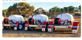
The design incorporates a tandem axle that has been designed to maximise stability and weight distribution for easy access to differing terrains like sand and gravel, and easy maneuverability in urban areas.
