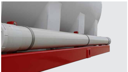
3-inch Delivery Hoses in PVC Holders (both sides)
